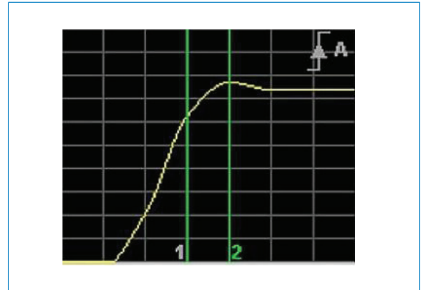
Figure 3b. Waveform analysis with time 10 ns/div time base and 1 sample per division.
